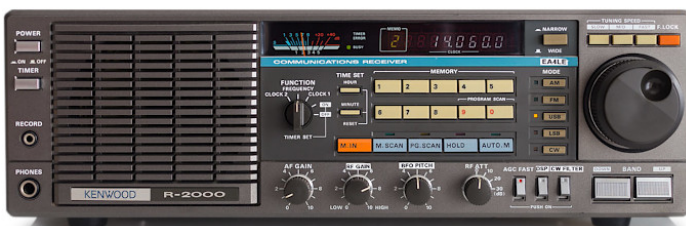
Figure 1: The Kenwood R-2000 was the first modestly priced communications receiver to offer a host of advanced capabilities; succeeding the R-600 and R-1000 . The Kenwood R-2000 is an all-mode SSB, CW, AM, FM receiver that covers 150 kHz - 30 MHz in 30
