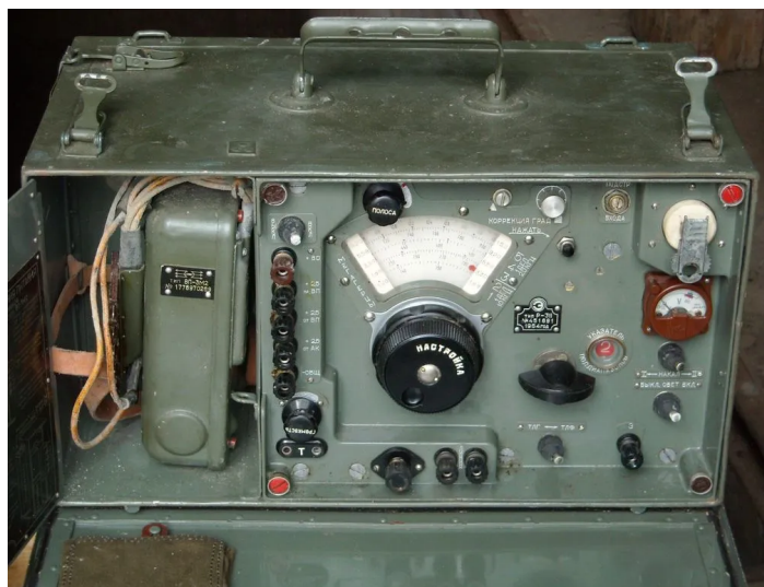
Figure 6: High Frequency radio receiver R-311 "Omega" was a Soviet shortwave radio for military use. Although it had a carrying handle, it wasn't really a portable set.
