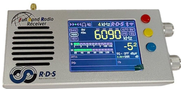
Figure 5: One of the emerging radios with the TEF-6686 chipset that are entering the marketplace.
