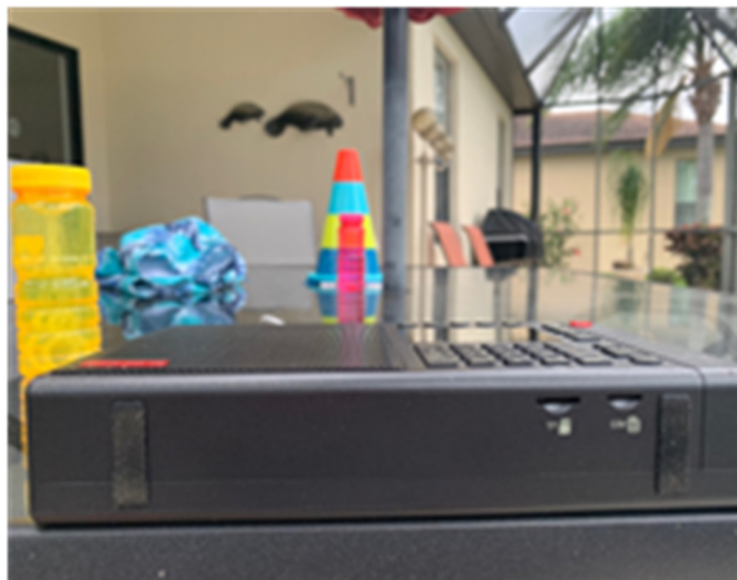
The base of the Choyong LC90 with receptacles for a TF card to play personal music and a SIM card to access internet radio via cellular.
