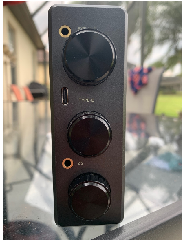
The right side of the Choyong LC90. Knobs from top to bottom: Tuning, Fine Tuning, Volume. Receptacles for External Antenna. Type C charging of the internal battery, Ear or Head Phones. The left side of the radio has no knobs, switches or receptacles.
