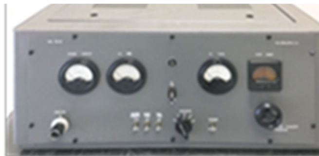
Hallicrafters HT-9 transmitter built from 1939. With interchangeable tuning units, the 54 kg device could work on different wavebands. The device on Swan was set up for the 14 MHz range. Transmission power CW 100 watts, language 75 watts.
