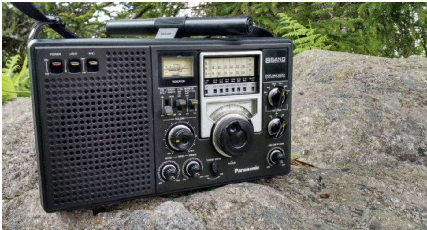
Or in the case of the Panny RF-2200, use its steerable ferrite bar antenna!
