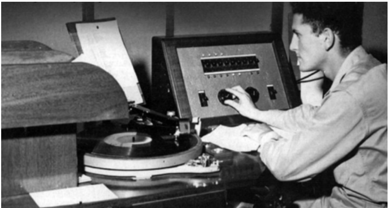
A typical broadcast package: note the simple mixer and a turntable that pulls double-duty — able to cut or play back discs.
