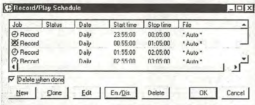
Figure 7. This window is used to manage multiple timed recording operations. No keyboard operations are required to Enable/Disable or Edit various individual timed recording sessions. The Clone function is quite useful when establishing repetitive timed recordings.
