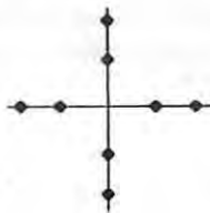
Figure 1: A signal with this phase/amplitude structure is called 8 QAM because it has the ability to signify 8 different states.
