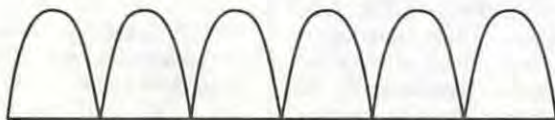
Figure 3. Distorted Envelope of Standard Full Carrier SSB at 67% Modulation with Sine Wave Single Tone Modulation. Distortion is 23% using Envelope Detector.
